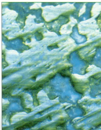
Magnified view of cured resin sealing porosity in a metal part.
