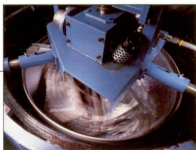
Parts immersed in resin wet vacuum cycle begins
