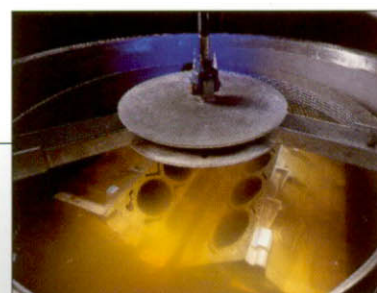
Parts are then submerged in Activator Solution to initiate cure
